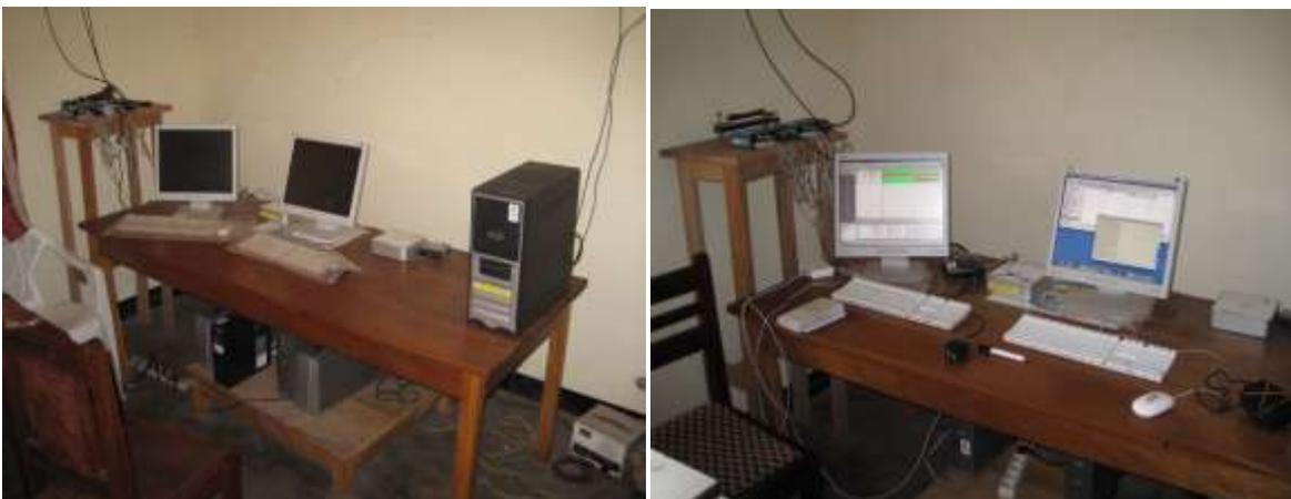
**Figure 25: Servers at GVO: master radios are visible on the high table to the left of the computers used for data acquisition and ftp servers. UPS and the power rectifier/inverter are below the table.**
