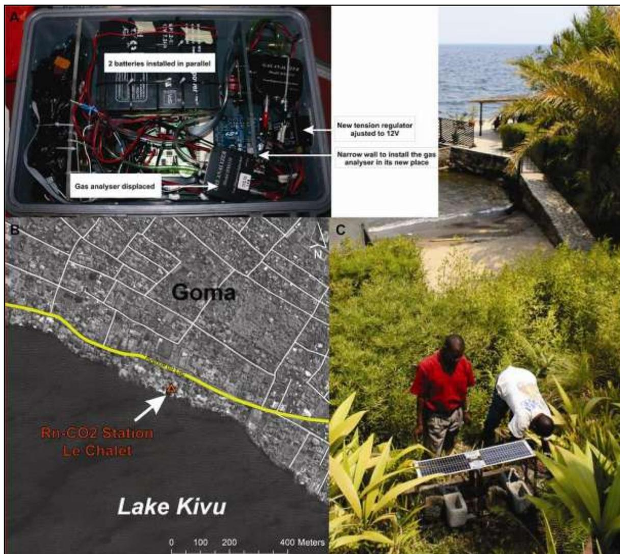
**Figure 39: installation of the CO<sub>2</sub>-Rn continuous measuring station in “Le Chalet”, Goma. A = major changes inside the instrument during the August 2009 maintenance. B = Location of the station “Le Chalet”. C = Solar panel installation.**
