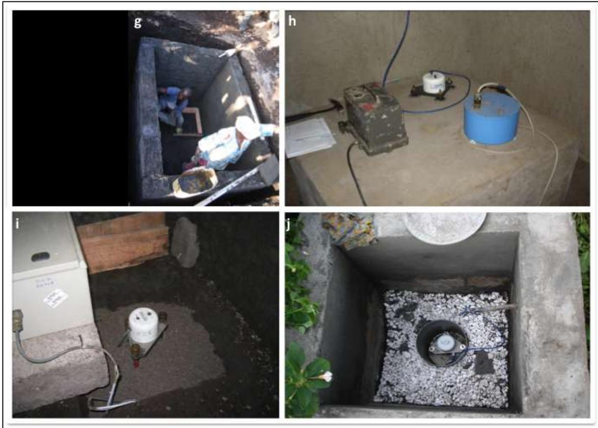
As evidenced here, such type of site represents a significant investment of time and energy. Another important aspect to be taken into account is the time during which the instrument is expected to remain. Tilt measurements are meaningful if they are recorded during a sufficiently long period – typically months or years – in order to identify the seasonal effects or the meteorological influences...
